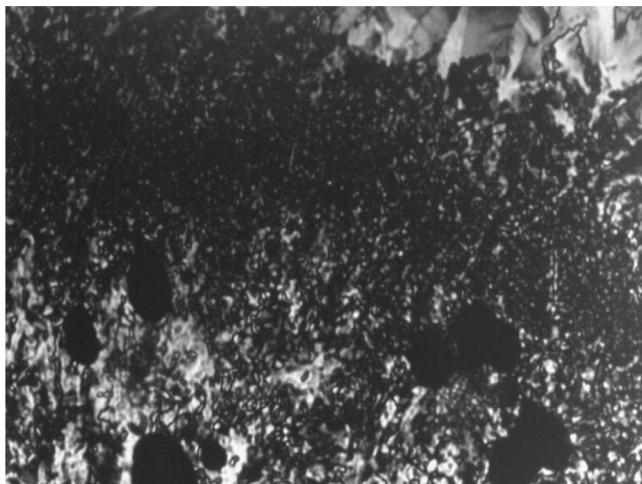
FIGURE 5 Polarizing optical micrograph of compound VII with TNF CT-complex on cooling, contact preparation, at 24.0°C, \times 250 .
